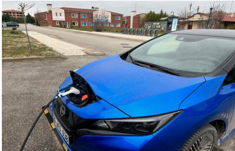
Figure 36 A view of the V2G compatible vehicle during charging process
