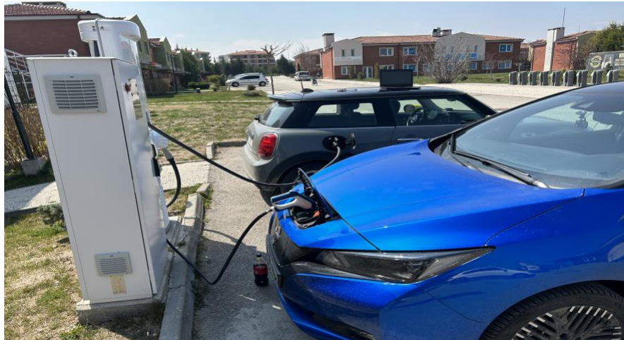
Figure 45 Simultaneous testing of V2G and V1G compatible vehicles
