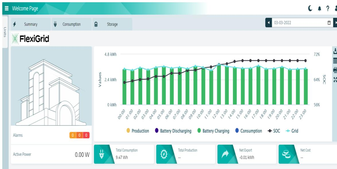
Figure 28 Web Interface of the battery management system
