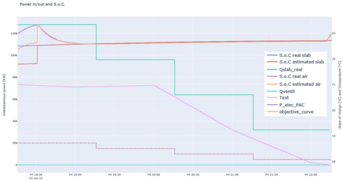
Figure 36: Example of thermal MPC controlling the heat pump electrical power and the power provided by the ventilation units
