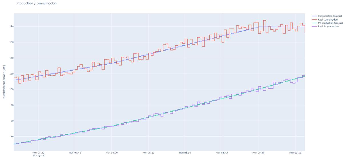
Figure 32 : Example of forecasted consumption / production vs actual value
