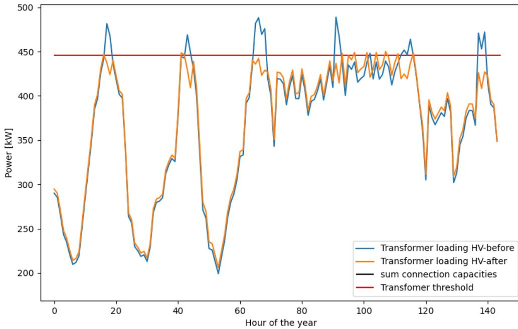
Figure 3-14 Transformer loading at RO before and after market activation- "impact-based" demand curve market clearing
