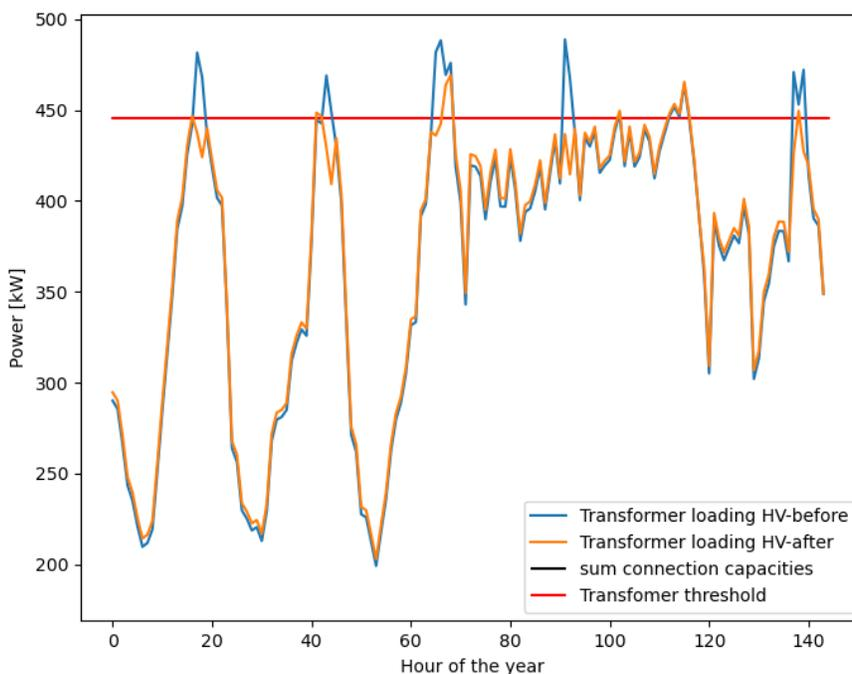
Figure 3-16 Transformer loading at R0 before and after market activation- “probability-based” demand curve market clearing
