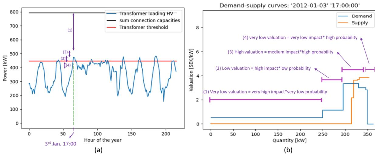
Figure 3-9 A "probability-based" demand curve of a capacity-limit cap product. (a) illustration of the different valuation parts of a demand curve on the loading forecast plot, (b) illustration of the different parts of a "probability-based" demand curve. The numbers for valuations are arbitrary values used only for illustration purposes.
