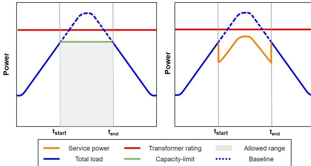
Figure 3-1 Baseline-based (on the right) and capacity-limit based (on the left) flexibility products [13]
