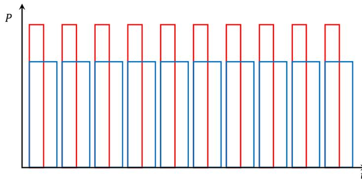
Figure 2-2 Constant power load's reaction to voltage drop
