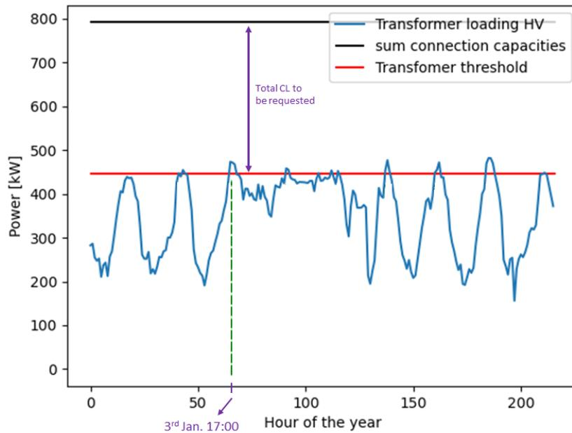
Figure 3-7 Transformer loading forecast for a period of 10 days. CL refers to the capacity-limit cap product to be requested.
