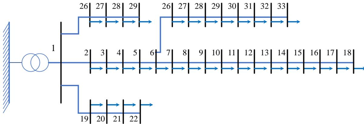
Figure 2-1. 33-Bus IEEE Standard Test System
