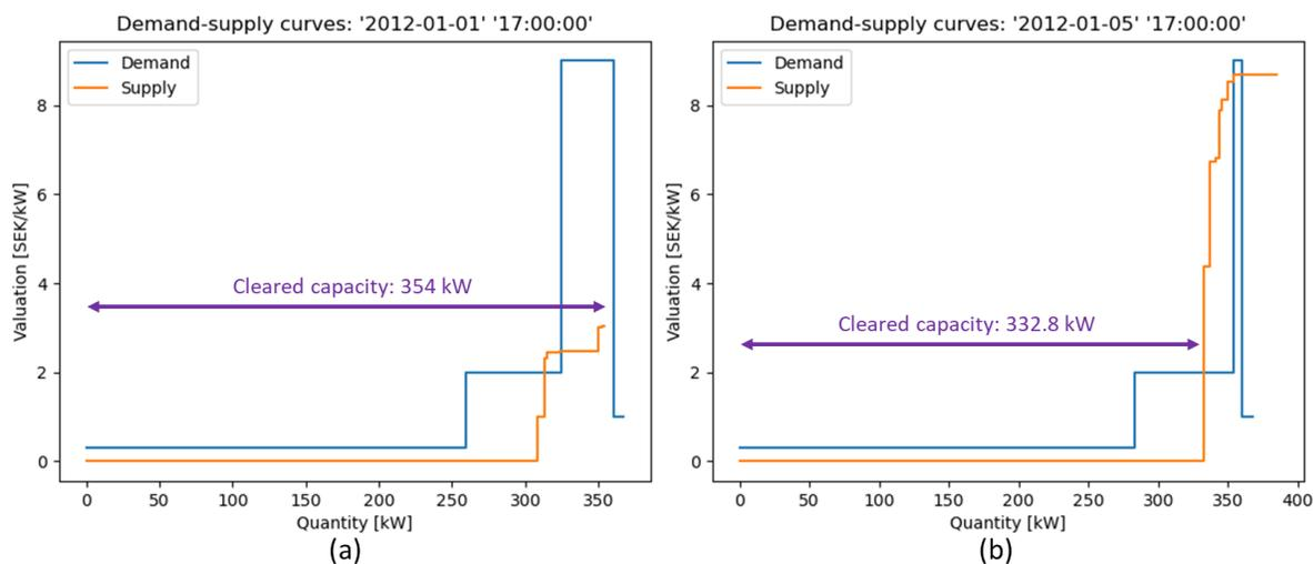
Figure 3-15 Two hours as examples for the supply-demand curves and the cleared capacities- “probability-based” demand curve market clearing
