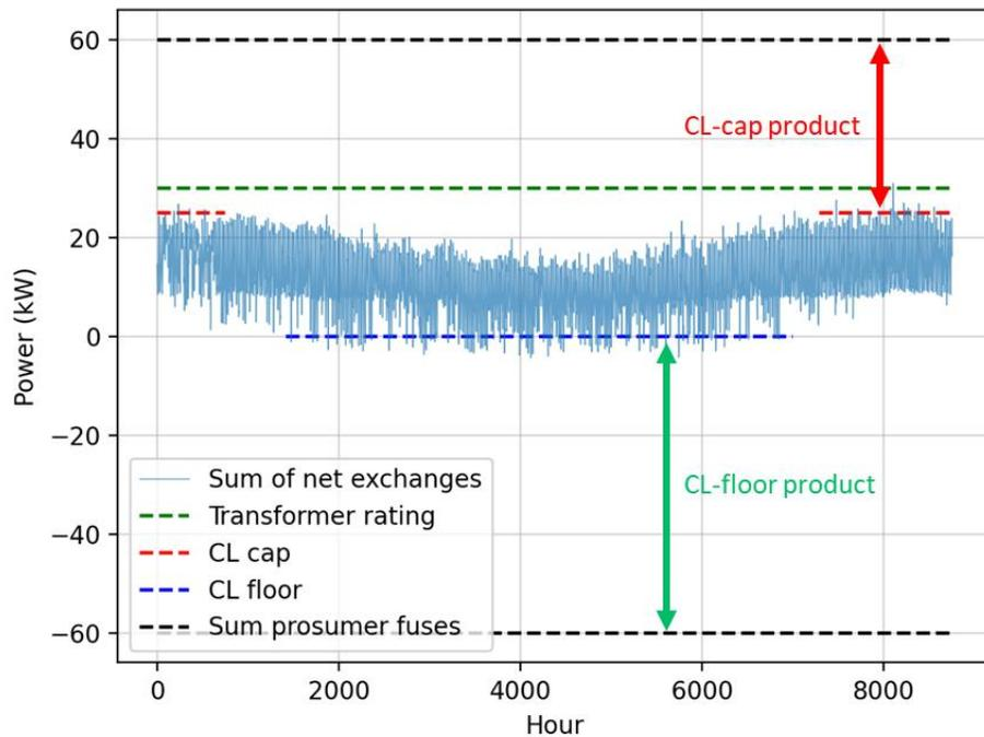
Figure 3-4 Capacity-limit cap, and capacity-limit floor products
