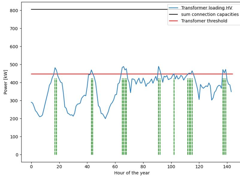
Figure 3-12 The loading of the transformer at bus R0. The green dashed lines represent the hours with loading over the transformer threshold. The threshold is assumed to be 95% of the transformer’s rating.
