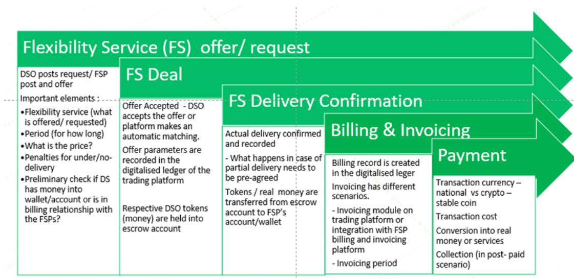
Figure 2-4 Flexibility services (FS) trading process
