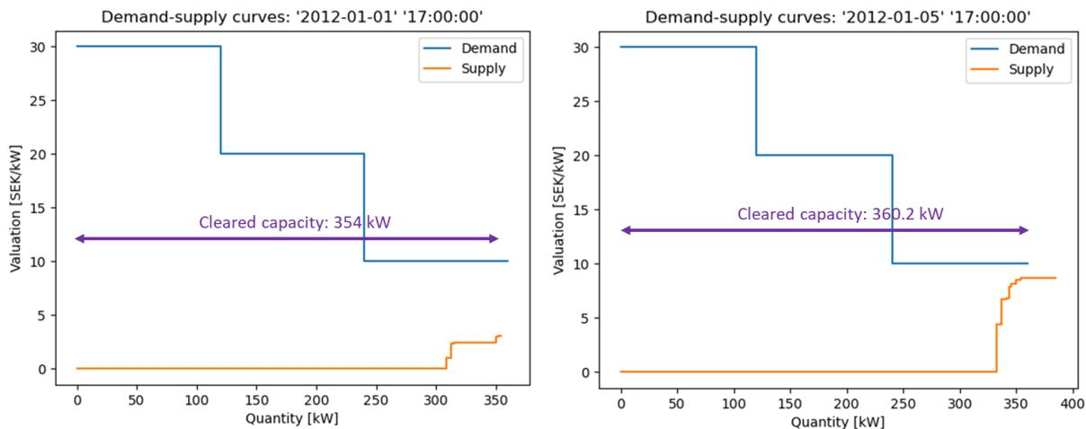
Figure 3-13 Two hours as examples for the supply-demand curves and the cleared capacities- “impact-based” demand curve market clearing
