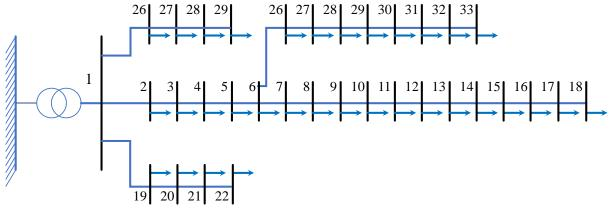
Figure 2-1. 33-Bus IEEE Standard Test System
