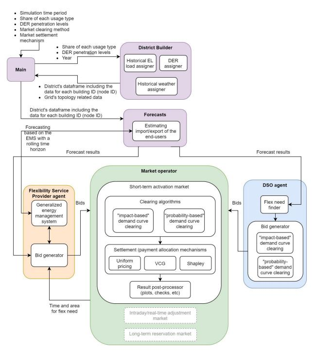
Figure 3-10 Overview of the model modules
