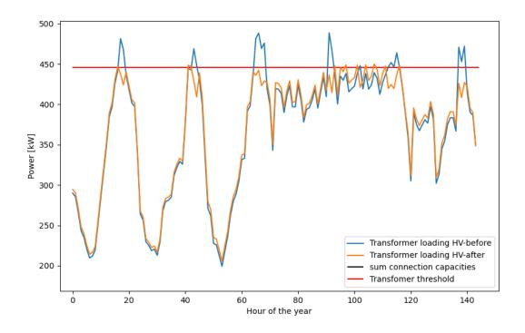
Figure 3-14 Transformer loading at R0 before and after market activation- "impact-based" demand curve market clearing
