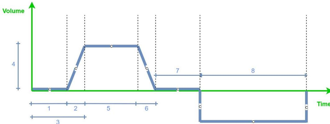
Figure 12 Energy product characteristics (modified figure from [66] and [69]). 1: Preparation period, 2: Ramping period, 3: Full activation time, 4: Min and max activation quantity, 5: Min and max delivery period, 6: Deactivation period, 7: delay period, 8: payback period
