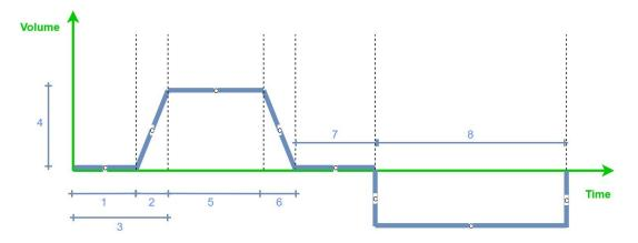
Figure 12 Energy product characteristics (modified figure from [66] and [69]). 1: Preparation period, 2: Ramping period, 3: Full activation time, 4: Min and max activation quantity, 5: Min and max delivery period, 6: Deactivation period, 7: delay period, 8: payback period
