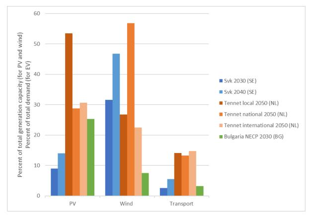
Figure 9 Comparison of distributed generation and transport as a share of total installed capacity or total electricity demand. SE: Sweden, NL: The Netherlands, BG: Bulgaria
