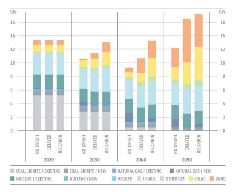
Figure 7 Expected installed generation capacity in Bulgaria for the three SEERMAP scenarios [23]
