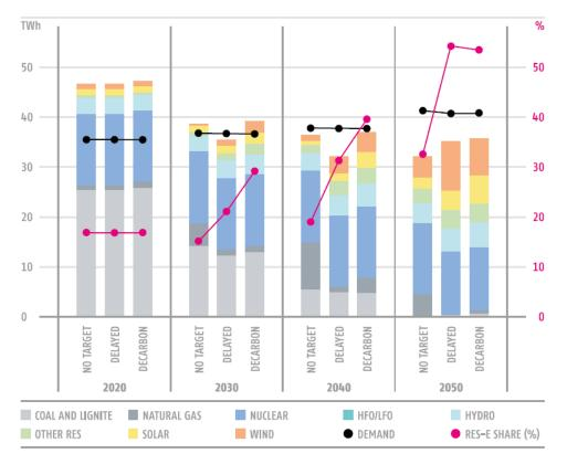
Figure 8 Expected electricity production from different sources of electricity demand in Bulgaria for the three SEERMAP scenarios [23]
