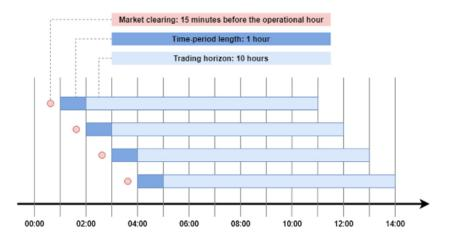
Figure 13 Rolling time-horizon clearing in FED-EM (adopted from [73])
